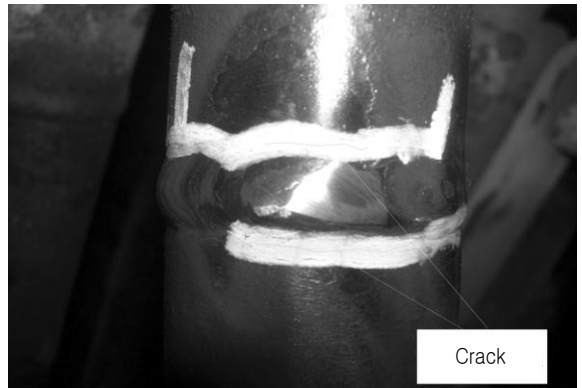
(a) Longitudinal crack and heated affected zone crack Crack
