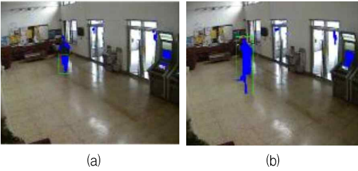
Fig. 2. (a) Object detection without morphology post-processing technique (b) Object detection with morphology post-processing technique
