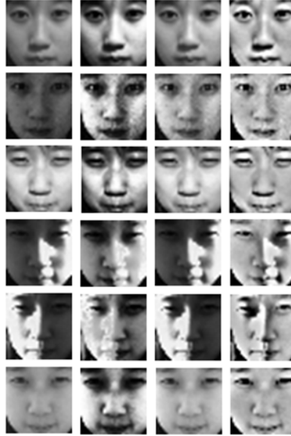
Fig. 10. The face images with illumination normalization (a) original image (b) with histogram equalization (c) with histogram stretching (d) with the Retinex filter
