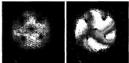
(a) Amplitude (b) Phase Fig. 7 Composite Multizeros Optical Beam Produced by Superposing the Two Beams with n=5 and n=1
