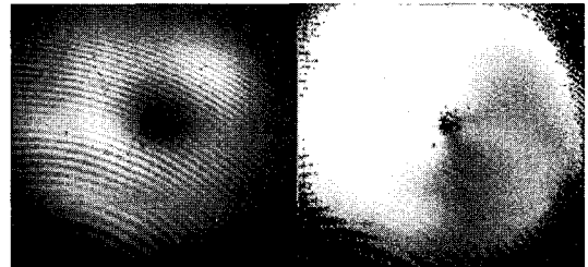
(a) Amplitude (b) Phase Fig. 6 Multizeros Optical Beam with n=1 after Propagation
