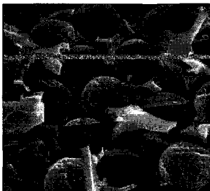
Fig. 3 Cross-sectional view of re-impregnated CFRP samples.
