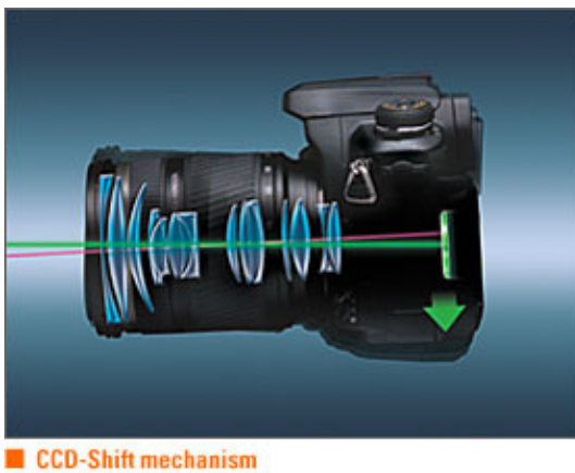
Fig. 2. The CCD-Shift Mechanism [8]
