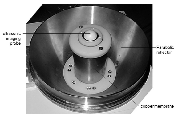
Fig. 8. A photograph of the cylindrical electromagnetic shock wave transducer [30].
