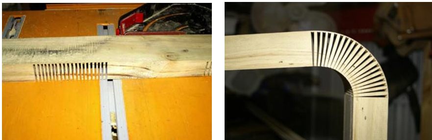
Fig. 8. Kerf bending process.
