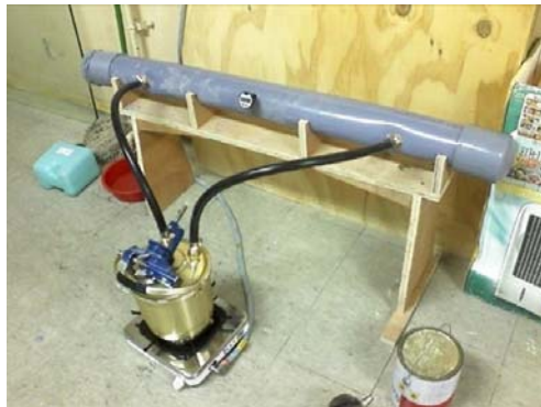
Fig. 3. steam box for wood bending.
