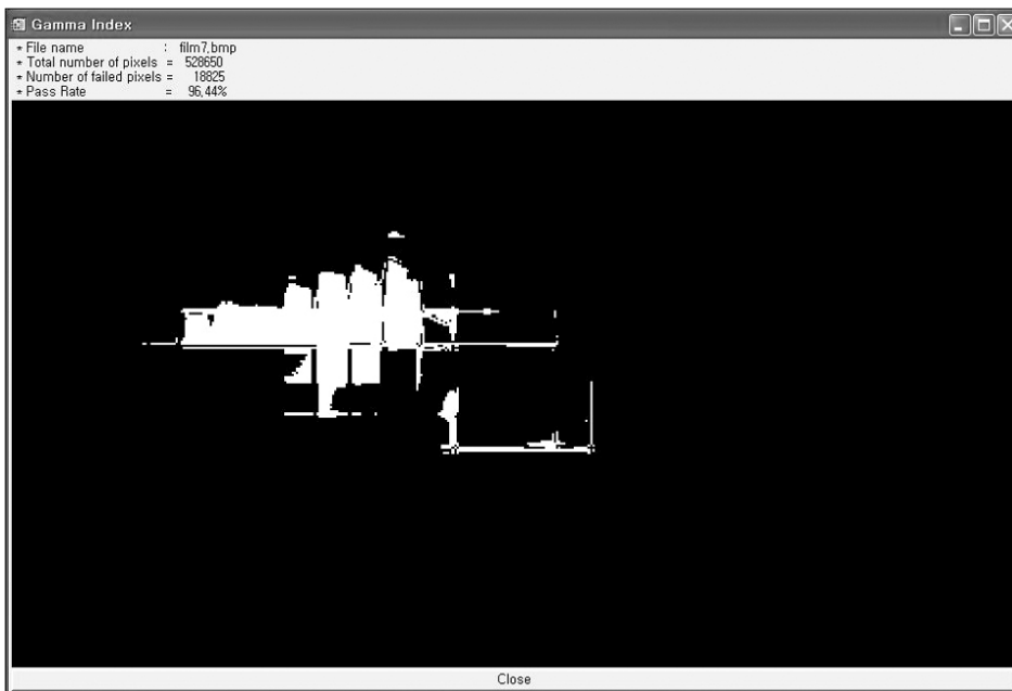
Fig. 4. The result of the PassRT program. The two-dimensional distribution of gamma index for the Field# 7 of the film measurement was analysed by the program.
