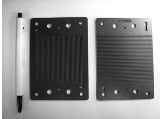
Fig. 1. Pictures of compression-molded carbon composite bipolar plate. Gas channel(left) and cooling line(right).
