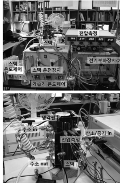
Fig. 4. Stack operation system(up) and PEMFC stack(down).
