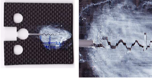
Fig. 6 Fatigue crack growth behavior at the surface of 0°/90° CFRP specimen
