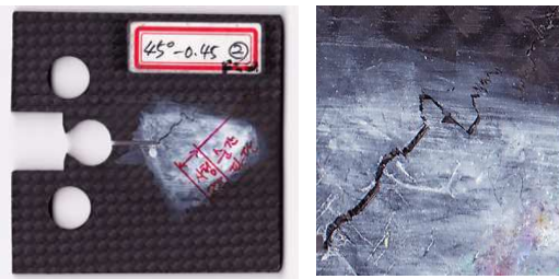
Fig. 7 Fatigue crack growth behavior at the surface of 45°/-45° CFRP specimen
