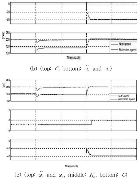
**Fig. 3** Simulation response in the back-EMF constant decreased by 30% with the load variation (200rpm, 0→2Nm,  $\hat{K}_e = 0.7K_e$ )
