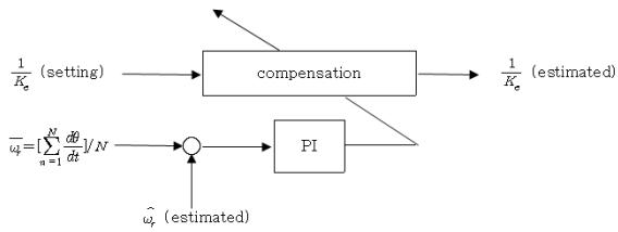
Fig. 1 Block diagram of back-EMF constant compensation
