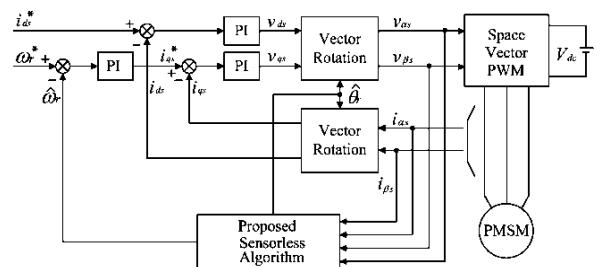
Fig. 2 Configuration of overall system
