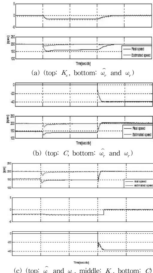
**Fig. 4** Experimental responses in the back-EMF constant decreased by 30% with the load variation (200rpm, 0→2Nm,  $\hat{K}_e = 0.7K_e$ )
