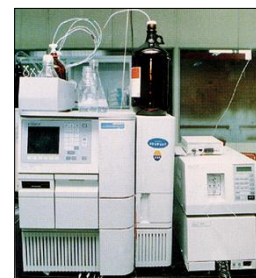
Fig. 3 HPLC spectroscopy for analysis of furan compounds
