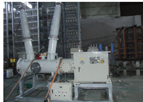
Fig. 6. Testing facility and 145kV 40kA GCB.
