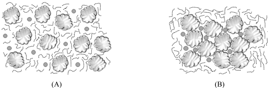
Fig. 11. (a) Electrostatic stabilization and (b) depletion flocculation of CMC coating colors.
