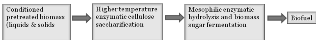
Fig. 2. Hybrid Hydrolysis and Fermentation (HHF).
