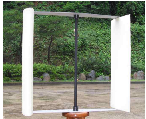
Fig. 8 Configuration of experimental VAWT model
