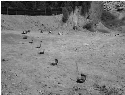
Fig. 4. Seismographs installed in the study area.
