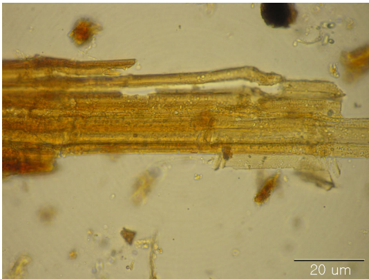
Figure 6. Dislocation of fiber.
