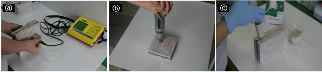
Figure 5. The verification of filling effects. (a) The sample images of the ultrasound exploration. (b) The sample measurement by Schmidt hammer. (c) The filler injection to the internal of the sample.
