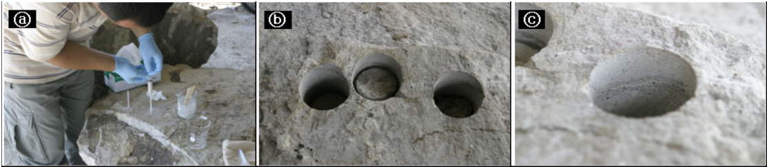
Figure 10. (a) Injection method of outcrop sample filler. (b) and (c) Checking the results of filling.
