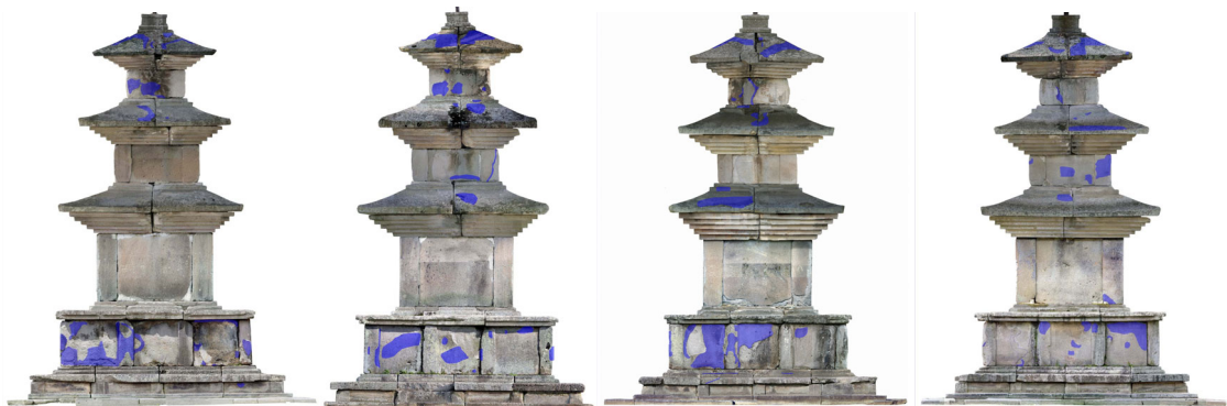
Figure 13. The range of opening pores for Three-storied Stone Pagoda at the West of Gameunsaji Site from the left to the east, west south, north side view.
