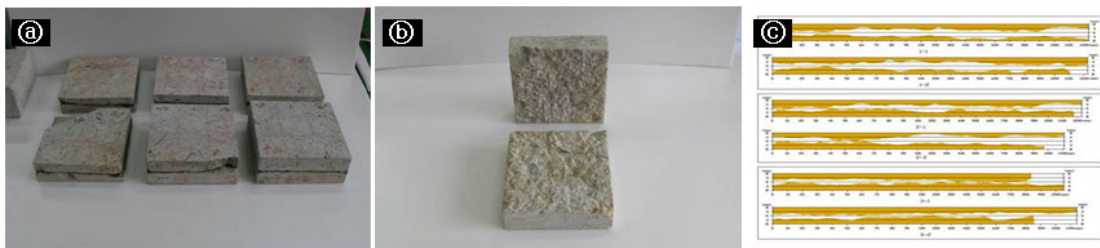
Figure 4. The sample is consists of dacitic tuff. (a) Producing samples for experiment, (b) The form of the sample internal opening, (c) The range of the sample internal opening.
