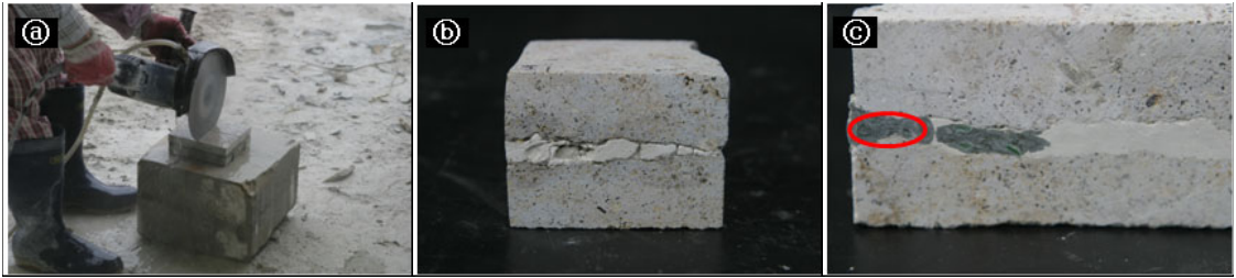
Figure 9. Checking the cross section of the sample after filling. (a) Sample cut, (b) Sample No. 5; semiliquid method, (c) Sample No. 1; injection method.
