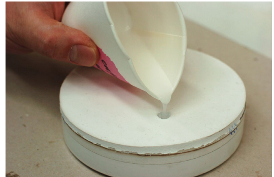
Figure 10. Process of filling with urethane polymer.
