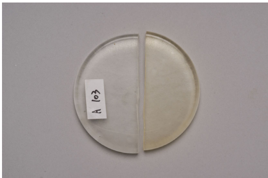
Figure 5. Color change of AW103, before and after UV exposure.
