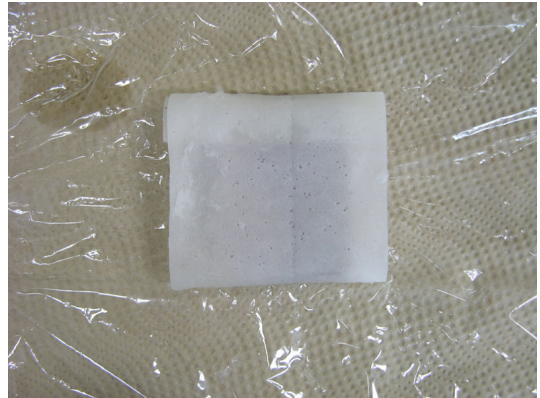
Figure 8. Wrapping with high absorption polymer.
