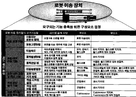
Fig. 2 Main/auxiliary components for configuration of robot transporting system
