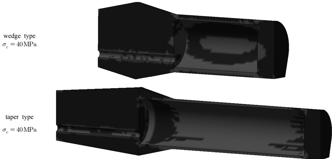
Fig. 6. FOS distribution in the plugs and concrete linings for p_i = 0 ; blue region (FOS>1), red region (FOS≤1)
