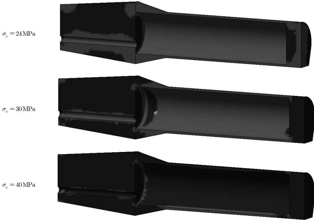
Fig. 5. FOS distribution in the taper shaped plug and lining; blue region (FOS>1), red region (FOS≤1)
