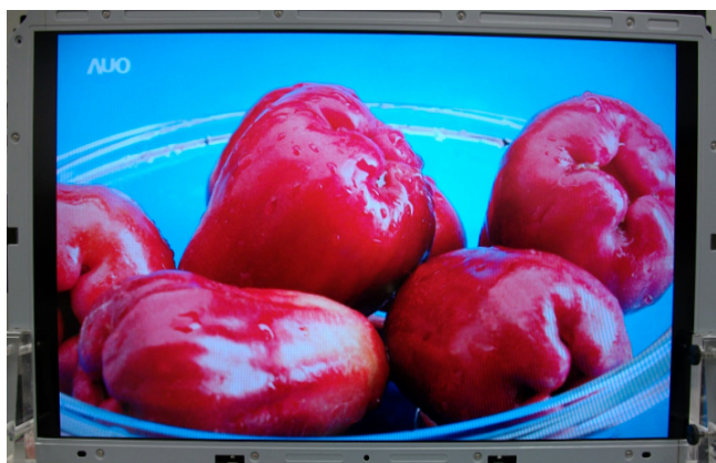
Fig. 7. A 32-inch IGZO TFT AMLCD.
