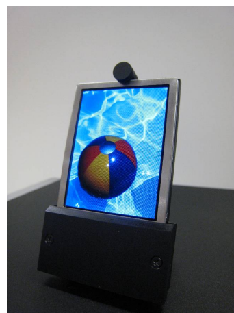
Fig. 5. A 2.4-inch IGZO TFT AMOLED with an inverted OLED.
