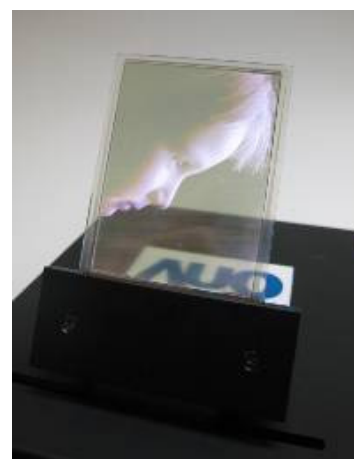
Fig. 6. A 2.4-inch IGZO TFT transparent AMOLED.
