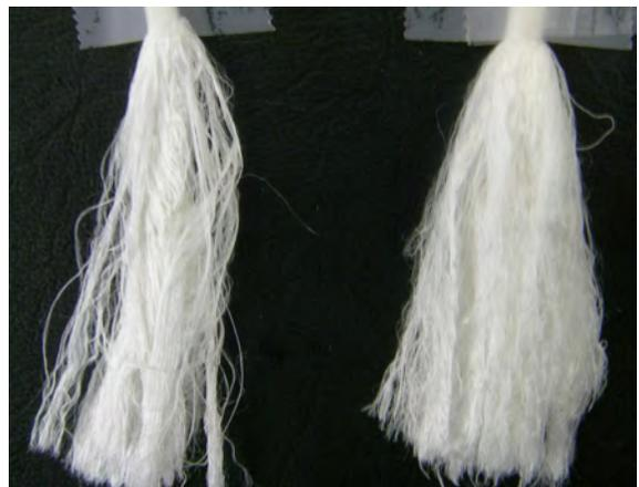
Fig. 7. Photograph of raw silk yarn bundles degummed at 80°C for 15 minutes(left) and 30 minutes(right) with 10%o.w.f. sodium carbonate.
