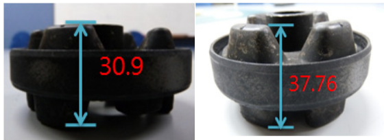
Figure 7. Normal insulator rubber height and noise occurred insulator rubber height.
