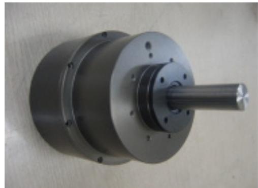
Figure 5: Overall picture of joint actuator
