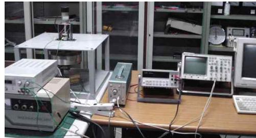
Fig. 6. Experiment apparatus for measurement of magnetization curve.
