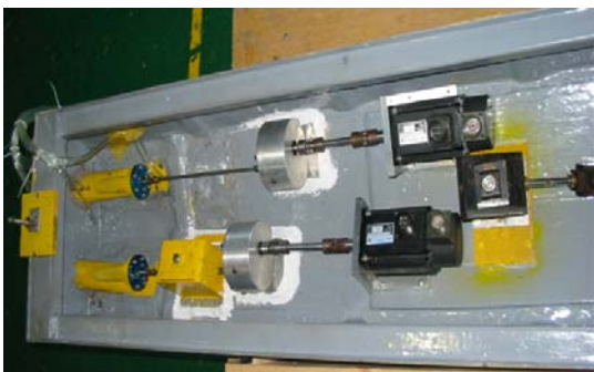
Fig. 4 Profile of Waterjet set-up in the model ship
