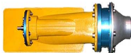
Fig. 3 Waterjet model with pressure tabs
