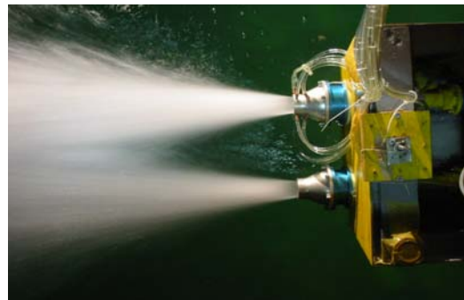
Fig. 6 Bollard test with pressure tabs
