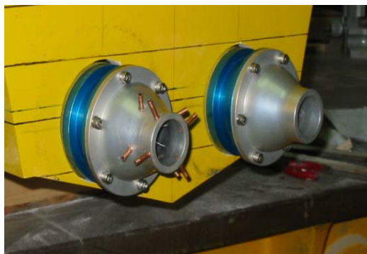
Fig. 2 Profile of model ship equipped with waterjet system
