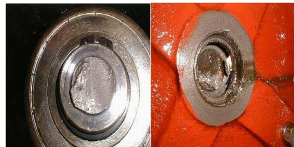
Fig. 3. Cross section of the failed shaft.
