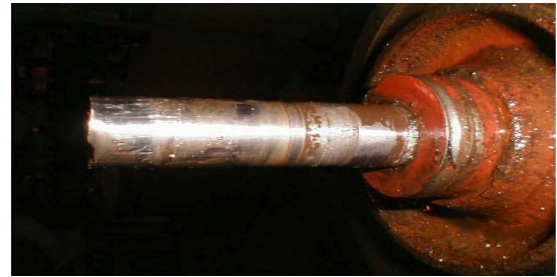
Fig. 1. Failure of the shaft.
