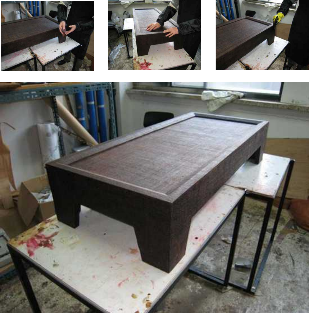
Fig. 20. Procedure for Making the Lower Portion of the Tea Table.
