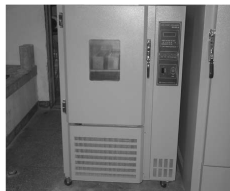
Fig. 2 Freezing and thawing test apparatus
