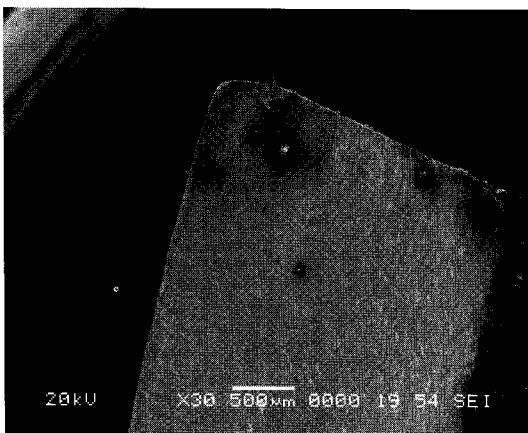
Fig. 5 Crack of low pressure compressor blade
