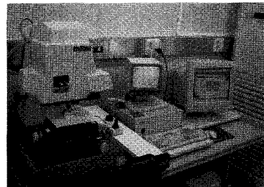
Fig. 2 Surface roughness measurement system (NT 2000)
