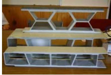
Fig. 2. Slab of FRP material.
