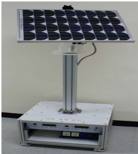
Fig. 8. Assembled sun-tracking power generation system.
