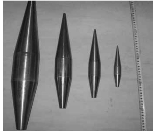
Fig. 10. Strikers for dynamic size effect research
