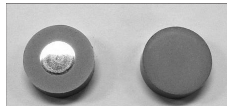
Fig. 2. Compacted bentonite block with copper & compacted bentonite block without copper.
