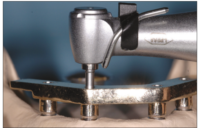
Fig. 4. Measurement of detorque values: Screw driver was carefully oriented in the long axis of the implant during screw tightening and loosening.
