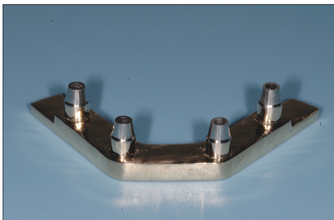
Fig. 1. Metal framework simulating a prosthesis that directly connected to four internal-connection implants.
