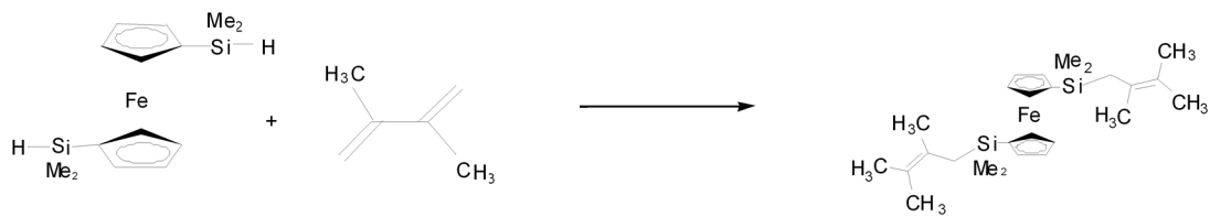
Scheme 4. Nickel catalyzed reaction of 1,3-dimethyl butadiene with 1,1'-bis(dimethylhydrosilyl)ferrocene
