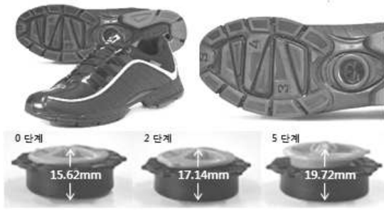
Figure 4. Testing shoe and arch support device
