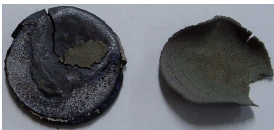
Fig. 4 Specimen degraded at 1,350°C for 50hr
