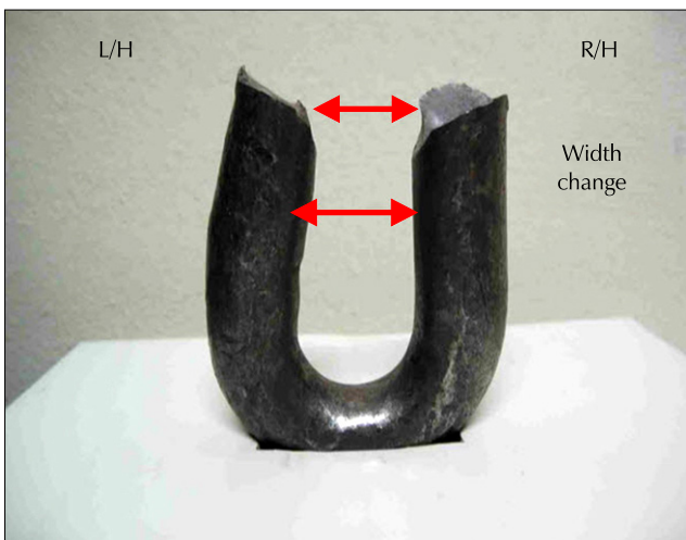
Fig. 2. Failed crane chain.
