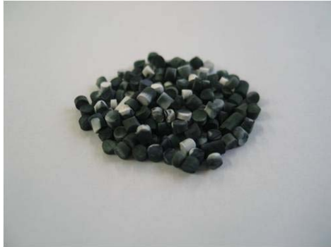
Fig. 11. Ru/Al 2 O 3 catalyst after the durability test for 2 hours
