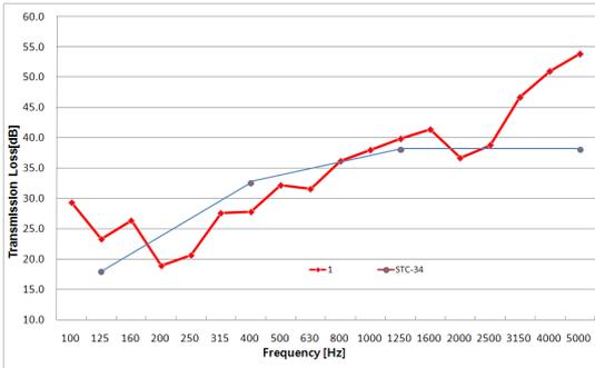
Fig. 4 Transmission loss of window part
