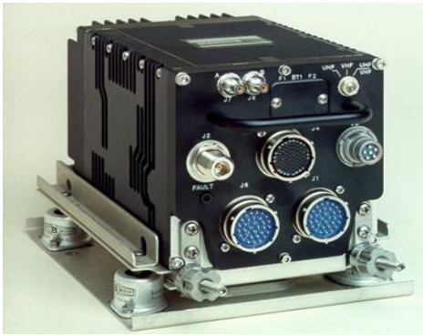
Fig. 2 Aerospace SRU with isolation mount
