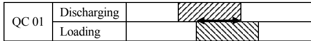
(b) Intervals for dual cycle operation performed by YTs serving the same QCs
