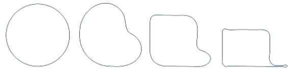
Fig. 4 Change of tube section during hydroforming process for the flanged tubular parts
