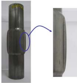
Fig. 13 Flanged tube part by experiment
