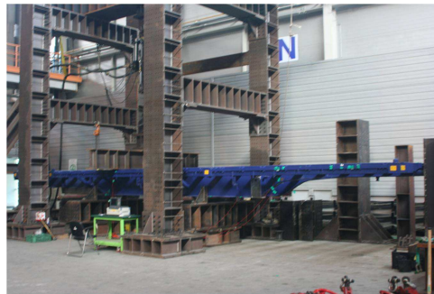
Fig. 12 Fatigue test on a prototype of the final optimized model
